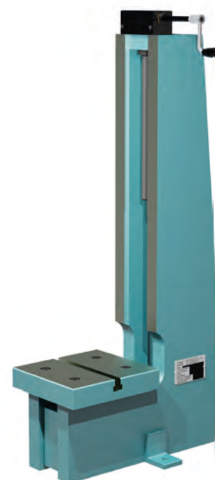
Example of a press frame with increased daylight
